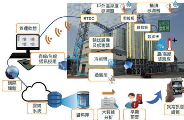
智慧型穀物倉儲與監控管理系統 Intelligent grain storage equipment and monitoring management system
