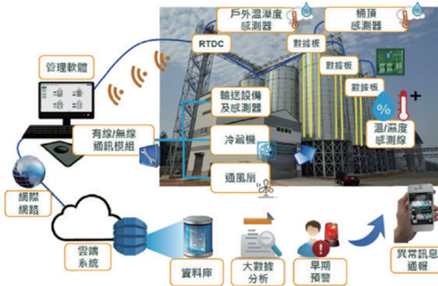
智慧型穀物倉儲與監控管理系統 Intelligent grain storage equipment and monitoring management system
